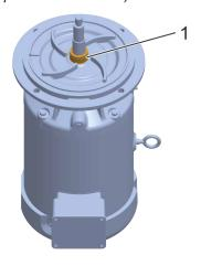
Fig. 111 Pushing the sliding ring into position (example: herborner.X-N)
