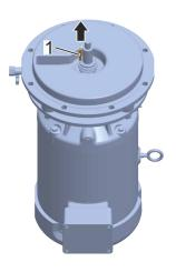
**15.** Remove the key (Fig. 71/1) from the motor shaft and put to one side for later assembly.
