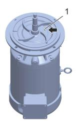
**5.** Tighten the locking screws of the mechanical seal (Fig. 112/1) evenly.
