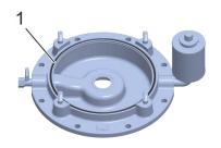
Fig. 90 Removing the O-ring (example: herborner.X-N)
