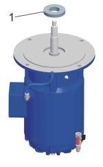
Fig. 48 Checking the shaft seal ring (example: herborner.X-N-C)
