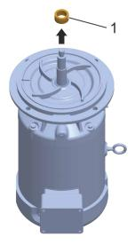
Fig. 92 Removing the sliding ring (example: herborner.X-N)
