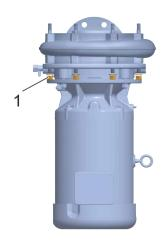
**11.** Tighten the nuts for fastening the pump casing together with the washers (Fig. 104/1).
