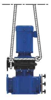
Fig. 23 Lifting points on the pump (example: herborner.X-N)
