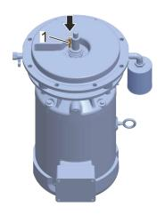
**10.** Fit the key (Fig. 117/1) into the slot on the motor shaft and press it fully down.
