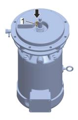
**5.** Fit the key (Fig. 99/1) into the slot on the motor shaft and press it fully down.
