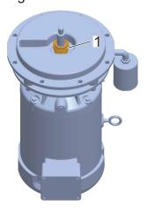
Fig. 116 Pushing the sliding ring with the spring into position (example: herborner.X-N)
