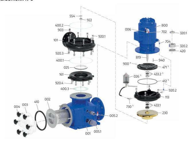
Fig. 136 Spare parts for herborner.X-N-C pump
