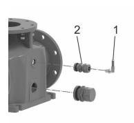
**6.** On the herborner.X-N-C, screw the return pipe into the upper screwed connection .
