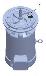
Fig. 91 Mechanical seal locking screw (example: herborner.X-N)
