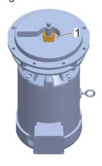
Fig. 98 Pushing the sliding ring with the spring into position (example: herborner.X-N)
