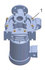
Fig. 61 Nuts for fastening the casing cover (example: herborner.F-N)
