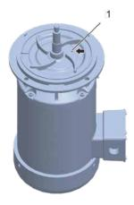
**5.** Tighten the locking screws of the mechanical seal (Fig. 100/1) evenly.
