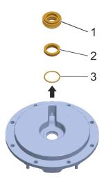
Fig. 60 Removing the mechanical seal (example: herborner.F-N/herborner.F-N-PM)
