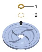
Fig. 78 Removing the stationary ring and o-ring
