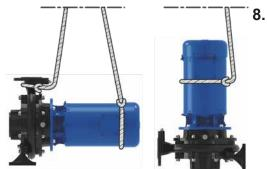
Fig. 119 Lifting points on the pump (example: herborner.F-N)
