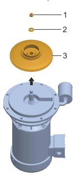
**32.** Remove the nut for fastening the impeller (Fig. 74/1) and the washer (Fig. 74/2) and place them to one side for later assembly.
