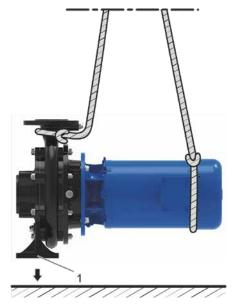
Fig. 23 Horizontal installation of the pump (example herborner.F-N)
