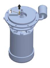
**34.** Remove the key (Fig. 75/1) from the motor shaft and put to one side for later assembly.
