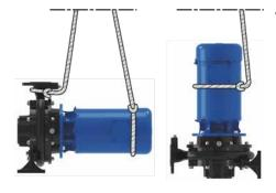
Attach the ropes, lashes or multi-point slings according to (Fig. 20.
