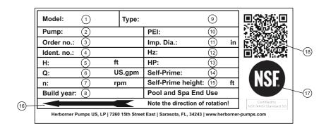
The name plate is located on the fan hood (herborner.F-N and herborner.F-N-PM) or the motor casing (herborner.F-N-C) and contains the following information:
