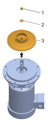
Fig. 56 Removing the impeller (example: herborner.F-N)
