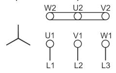
The 3 hp and 5 hp motors of the herborner.F-N-C are connected in a wye connection (Fig. 10) at the factory. The power supply is connected at terminals U1, V1 and W1.
