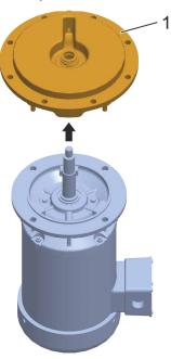
Fig. 59 Removing the intermediate casing (example: herborner.F-N)
