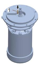
**5.** Fit the key (Fig. 88/1) into the slot on the motor shaft and press it fully down.
