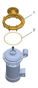
Fig. 65 Removing the pump casing (example: herborner.F-N)
