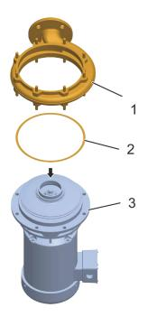
**9.** Place the seal (Fig. 92/2) on the intermediate casing (Fig. 92/3).
