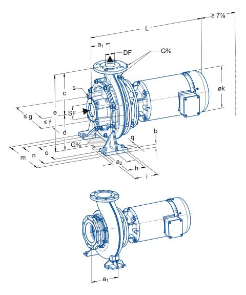
Fig. 120 Dimensions of herborner.F-N pump
