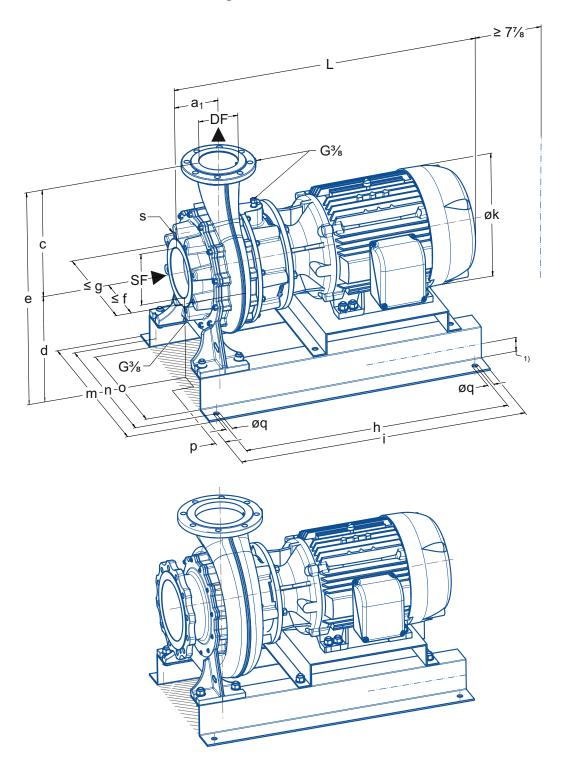
Fig. 121 Dimensions of herborner.F-N pump (version with base rail ≥ 50hp)
