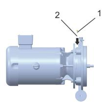
Fig. 109 Tightening the screw (example: herborner.F-N)
