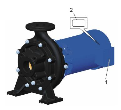
Fig. 34 Wiring the terminal box (example: herborner.F-N)
