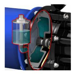
A fully-functioning Seal Guard system uses a media reservoir to prevent the mechanical seal from dry running for approx. two minutes. The media reservoir is automatically replenished by a supply container. This container can also be used to detect primary mechanical seal leakage.
