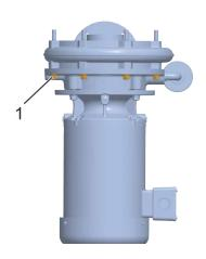
21. Remove the nuts for fastening the pump casing (Fig. 69/1) on all sides and place them to one side for later assembly along with the washers.
