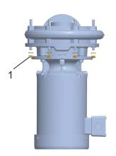
Fig. 88 Tightening the nuts for fastening the pump casing (example: herborner.F-N)
