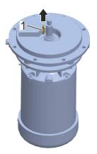
Fig. 57 Key in the motor shaft (example: herborner.F-N)
