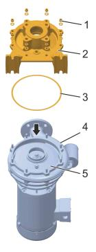
Fig. 107 Installing the casing cover (example: herborner.F-N)
