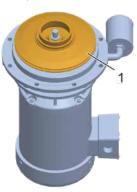
Fig. 101 Impeller pushed on (example: herborner.F-N)
