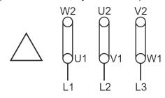
The motors of the herborner.F-N-C (except for 3 hp and 5 hp) are connected in a delta connection (Fig. 11) at the factory. The power supply is connected at terminals U1, V1 and W1.
