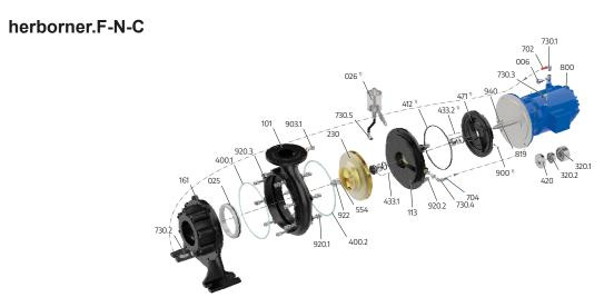
Fig. 117 Spare parts for herborner.F-N-C pump
