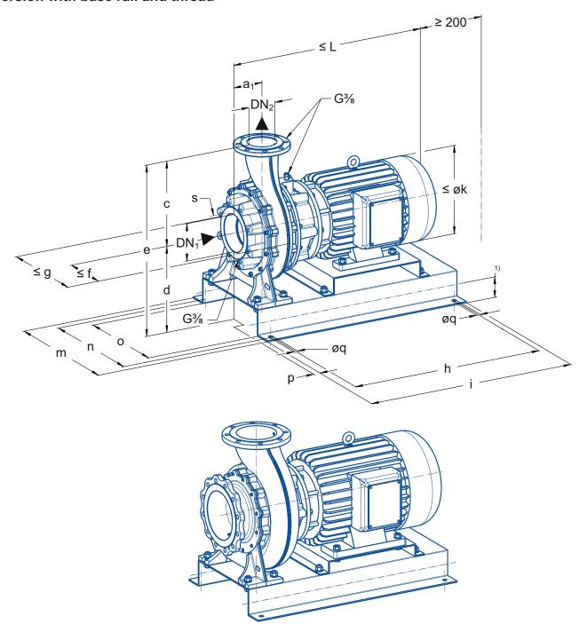
Fig. 123 Dimensions of herborner.F-N-PM pump (version with base rail ≥ 50hp)
