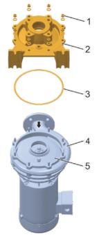
Fig. 90 Installing the casing cover (example: herborner.F-N)
