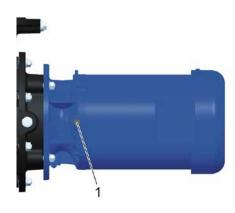
Fig. 42 Condensation water drain holes (example: herborner.F-N)
