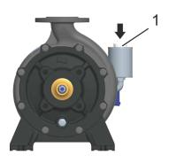
**24.** Refill the oil in the opening of the Seal Guard system compensation tank (Fig. 115/1) until it is half-full.
