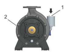
**22.** Add oil into the opening of the Seal Guard system compensation tank (Fig. 113/1) until the oil comes out from the opening of the screw (Fig. 113/2).
