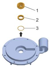
Fig. 73 Removing the mechanical seal (example: herborner.F-N/herborner.F-N-PM)
