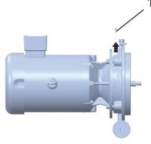
Fig. 67 Seal cover screw (example: herborner.F-N)
