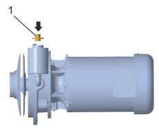
Fig. 66 Seal Guard system compensation tank cap (example: herborner.F-N)
