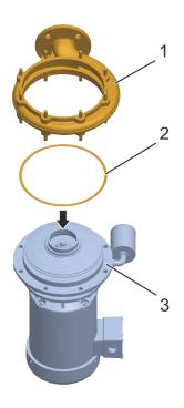
**14.** Place the seal (Fig. 109/2) on the intermediate casing (Fig. 109/3).
