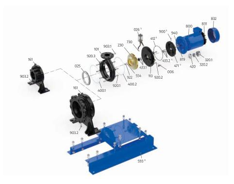
Fig. 116 Spare parts for the herborner.F-N/herborner.F-N-PM pump (example: herborner.F-N)
