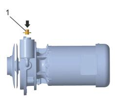
Fig. 111 Tightening the Seal Guard system compensation tank cap (example: herborner.F-N)
