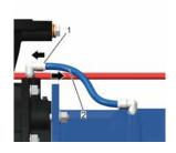
Fig. 49 Removing the cooling water pipe
