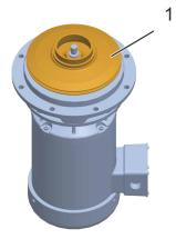
**6.** Push the impeller (Fig. 89/1) onto the motor shaft.
