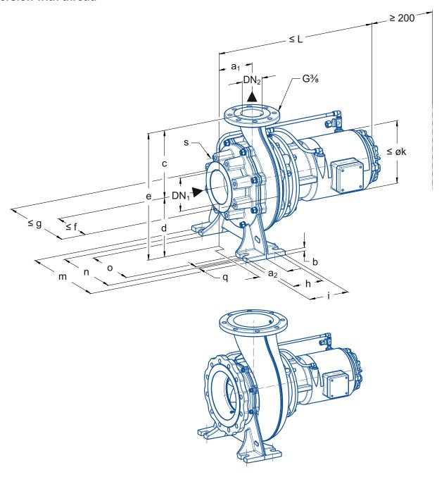
Fig. 124 Dimensions of herborner.F-N-C pump
