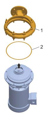
Carefully lift the loosened pump casing off the intermediate casing (Fig. 59/1).
