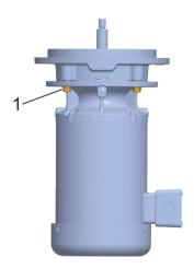
**13.** Remove the nuts for fastening the intermediate casing (Fig. 63/1) on all sides and place them to one side for later assembly along with the washers.
