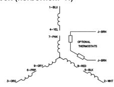
Numbering and wiring of the motor connection cables in wye connection (herborner.F-N)
