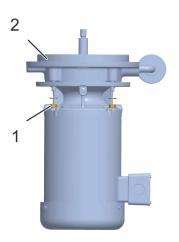
Fig. 98 Fitting the intermediate casing (example: herborner.F-N)
