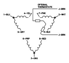
Fig. 6 Numbering and wiring of the motor connection cables in a delta connection (herborner.F-N)
