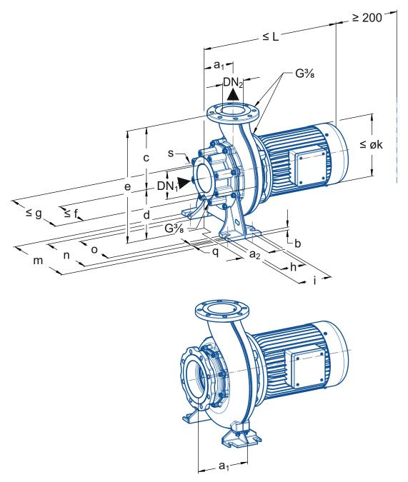
Fig. 122 Dimensions of herborner.F-N-PM pump
